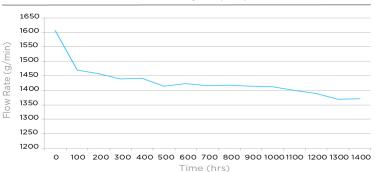
Testing was stopped at 1400hrs; the tubing was still functioning and mantained flow rate stability
