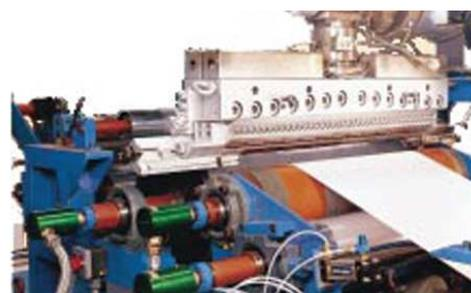
Orange overcoat masking tape on chill roll
