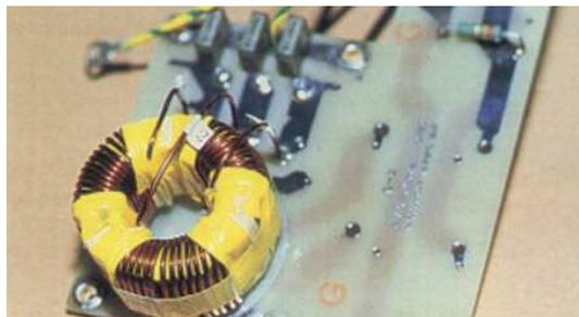
Coil outer wrap taping
