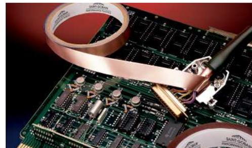
EMI-RFI copper tape shielding
