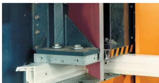
PVC extrusion welding, platen cover
